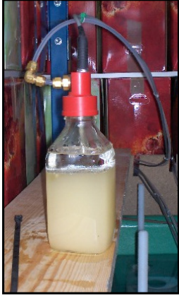
a SIMPLE SDD, containing 0.01-0.02 kg of C_2ClF_5 .
